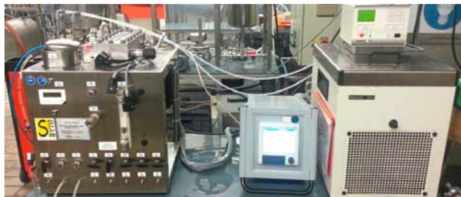
figure 3: Laboratory test unit Cube 80-VA (left) in the lab, with measurement box (middle) for acquisition and visualization of data and thermostat (right) (photograph: Chair for Food and Bioprocess Engineering at the Technical University of Munich (Weiherstephan site))
